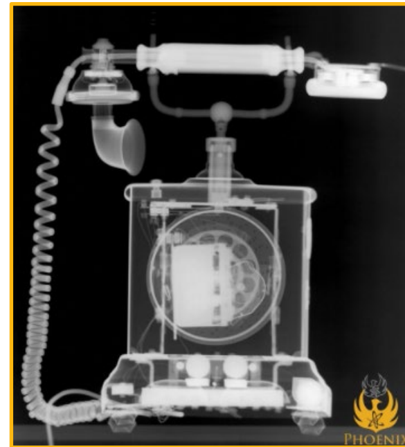
Neutron CT scan of rotary phone [3]
