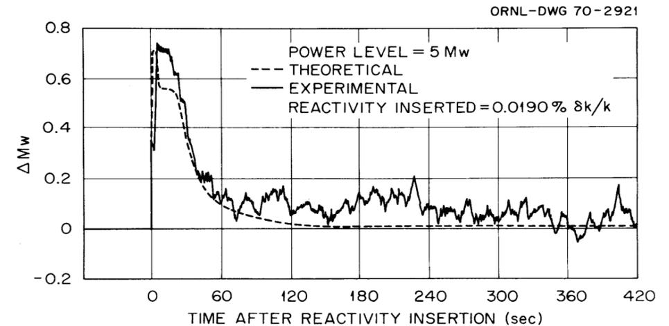
Fig. 3. Response of the Neutron Flux to a Step Change in Reactivity of 0.0190%  $\Delta k/k$  with the Reactor Initially at 5 MW.
