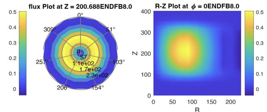
Fig. 4. Radial and axial planar view of the flux distribution modeled with ENDF/B-VIII.0.
