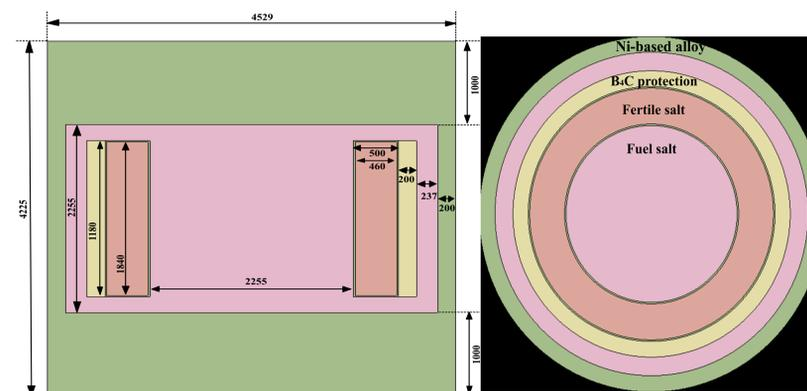
Fig. 3. Axial planar view (left) and radial planar view (right) of the MSFR core model (dimensions given in mm) [3].
