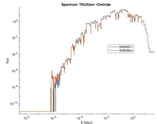
Fig. 5. Comparison of flux spectra with ENDF/B-VII.1 and ENDF/B-VIII.0 data libraries.
