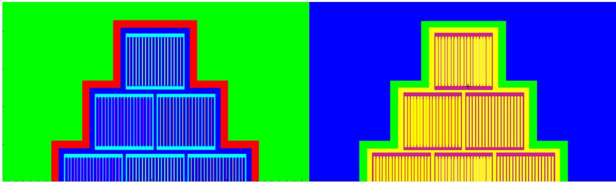
**Figure 3.** MPACT (left) and MCNP (right) models of NBSR-2 as rendered in VisIt and Xming, respectively. Reflective symmetry is observed along the right and bottom boundaries in each model.
