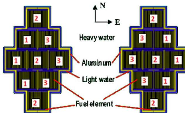
**Figure 1.** The current NBSR-2 core configuration.
