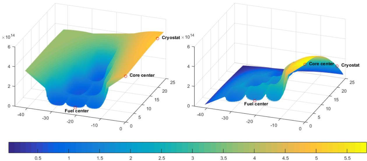
**Figure 6.** MPACT thermal flux from the full (left) and reduced (right) reflector models.
