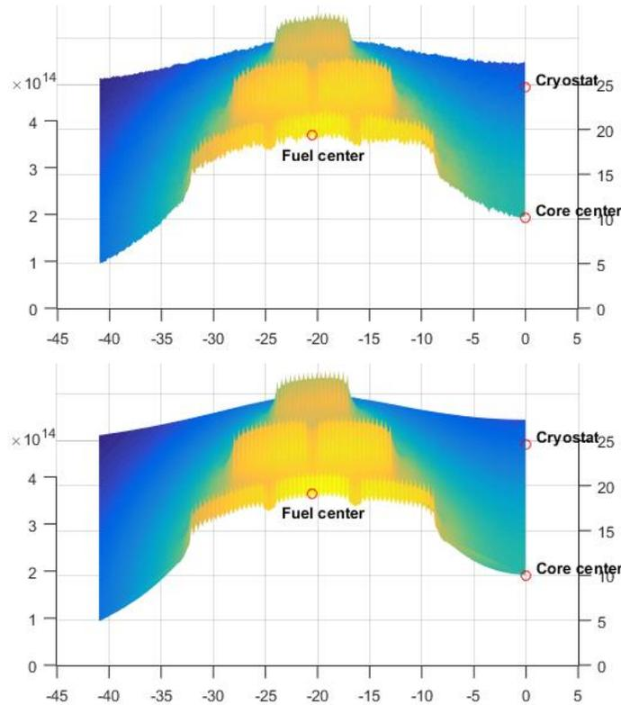
**Figure 4.** Fast flux in MCNP (top) and MPACT (bottom) with the full reflector model.
