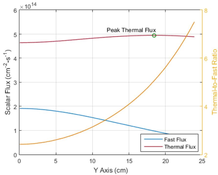
**Figure 5.** Flux and flux ratio profiles along the vertical centerline of the full reflector model, as calculated with MPACT using the full reflector model.
