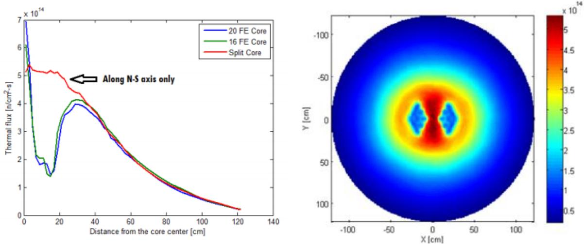
**Figure 2.** MCNP6 calculations for the thermal flux profile in NBSR-2 along the cryostat axis.
